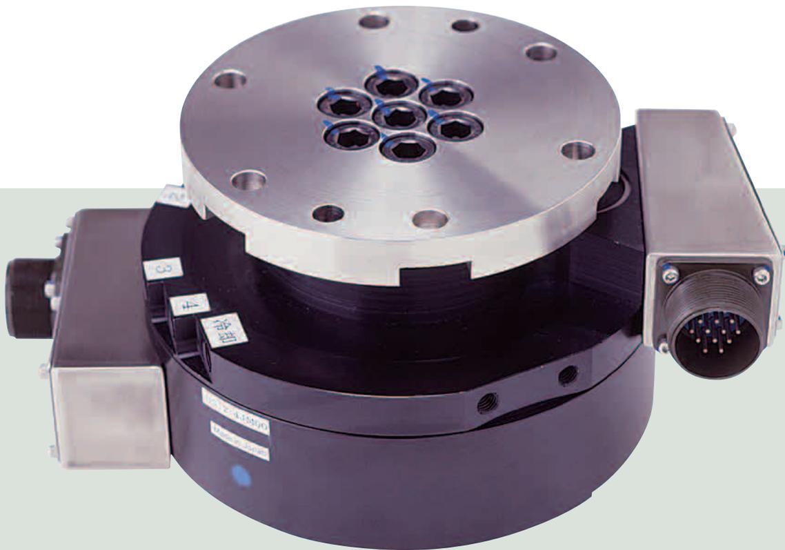
This unit integrates multi-contact signal communication channels required for material handling tooling applications. It talks to high-speed serial communication devices via a smoothly rotating disk. 150 kg payload robots and material handling equipment with equivalent capacity are the suitable applications for this unit. This unit can be adapted for "earth-grounded" applications as well, with optional contacts.
